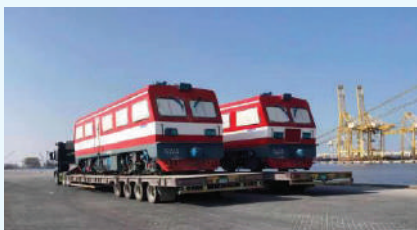
12M/15M LOW BED TRAILER 1200/1500X250X120CM L/C 40TON-60TON
