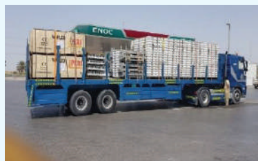
15M FLAT BED TAILER 1500X250X150CM L/C 25TON/40TON
