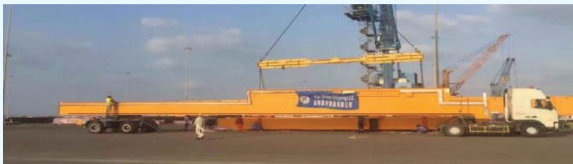
EXTENDABLE/DOLLY TRAILER LOAD UP TO 28M L/C 18TON-50TON
